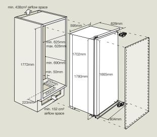
**Note:** Ventilation grille should be cut out to suit customer requirements with a minimum of 152cm² of cross-sectional area for ventilation grille airflow.
