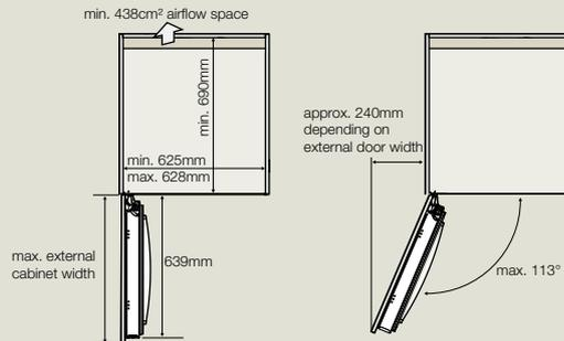
Note: Ventilation grille should be cut out to suit customer requirements with a minimum of 152cm² of cross-sectional area for ventilation grille airflow.
